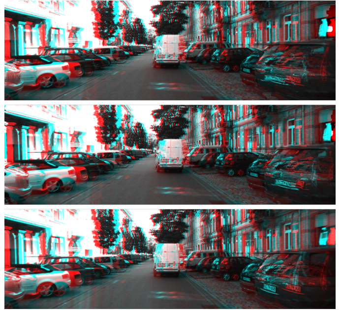
Fig. 12. 3D anaglyphs generated from the original left image and synthesized right view(top), synthesized left and right views (middle), and original stereo imagery (bottom)
