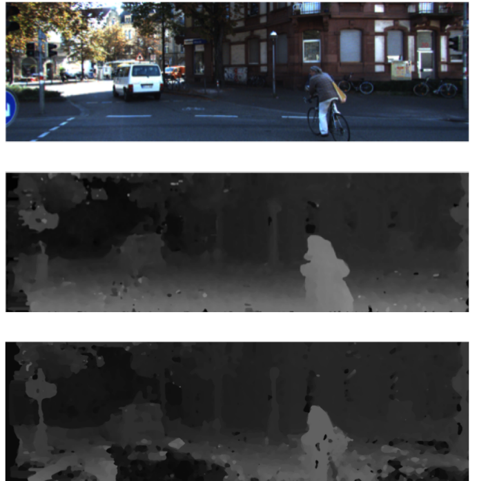
Fig. 9. (Top) the left image in the stereo pair.(Middle) disparity map created with the convolutional neural network. (Bottom) disparity map created with 9 \times 9 subtractive method.
