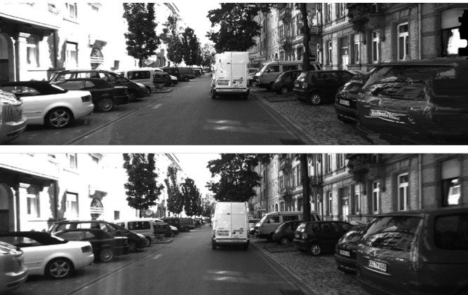
Fig. 11. A novel right view (top) is synthesized from the disparity map and a left image. The original right image is shown for comparison (bottom). Notice how much of the scene looks very natural such as the roads and buildings, but smaller features such as signposts are distorted.
