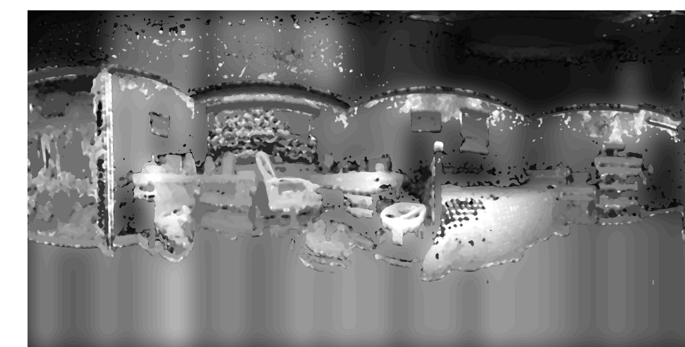
Pixel-level disparity map Brighter pixels correspond to greater pixel shifts i.e. closer objects.
