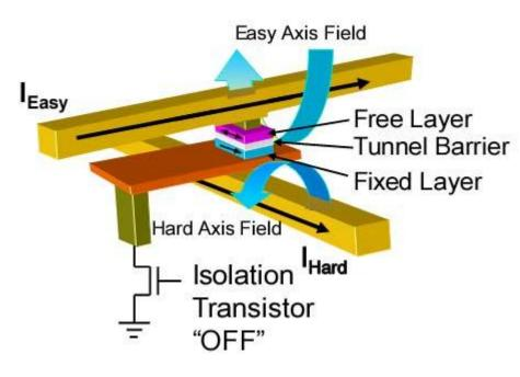
Transistor is "OFF" and current is passed through the write lines, an induced magnetic field is created at the junction, which alters the polarity of the free layer.
