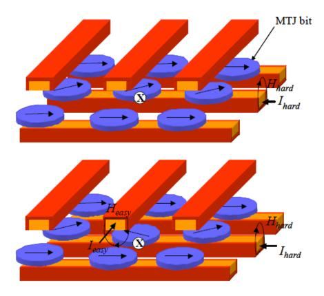
In order to change the polarity of the free layer, both fields are necessary.
